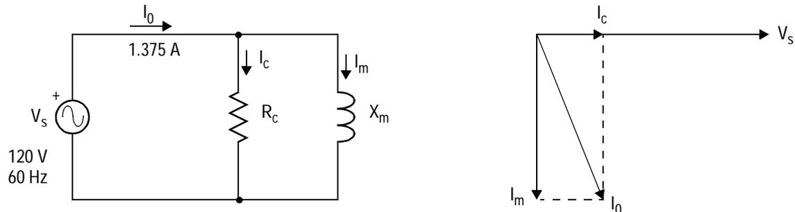
La réactance de la bobine 1:  $X_m = \omega L_1 = 120\pi \times 0.2356 = 88.83 \Omega$
