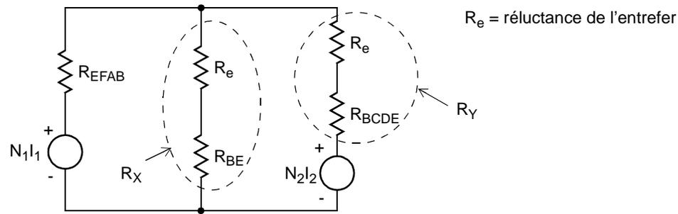
Réluctance de l'entrefer:  $R_e = \frac{e}{\mu_0 A} = \frac{0.5 \times 10^{-3}}{(4\pi \times 10^{-7})(2 \times 10^{-2} \times 3 \times 10^{-2})} = 6.6315 \times 10^5 \text{ At/Wb}$
