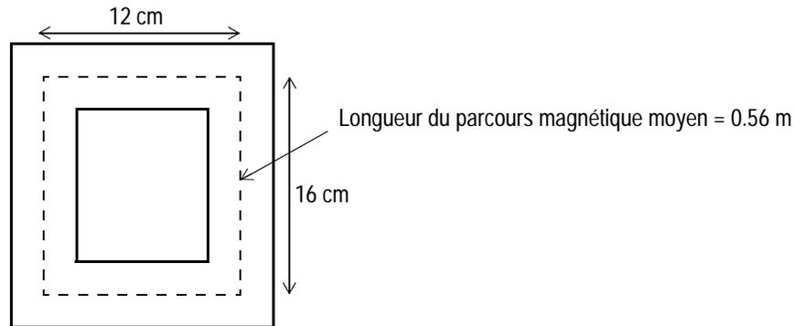
Réactance de la bobine 1:  $R_1 = \frac{l}{\mu A} = \frac{0.56}{2800(4\pi \times 10^{-7})(4 \times 10^{-2} \times 6 \times 10^{-2})} = 6.6315 \times 10^4 \text{ At/Wb}$
