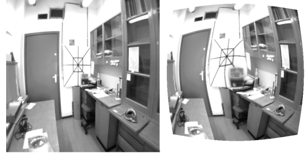
Figure 3: (a) the original image coming from the CCD (b) the same image after the remapping algorithm
