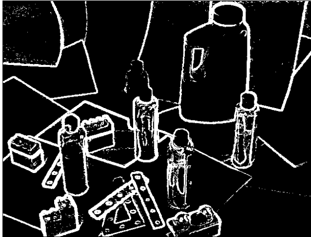
Figure 11: Difference Vector with intensity-based combined measure applied to the RGB space (offset=0.10 and slope = 75).
