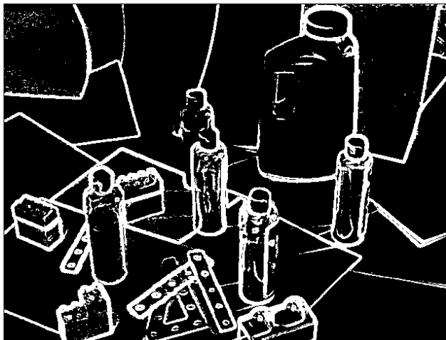
Figure 9: Difference Vector with saturation-based combined measure applied to the RGB space (offset=0.10 and slope = 75).
