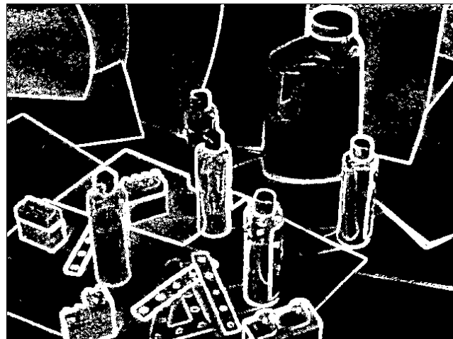
Figure 10: Vector Gradient with saturation-based combined measure applied to the RGB space (offset=0.25 and slope = 75).
