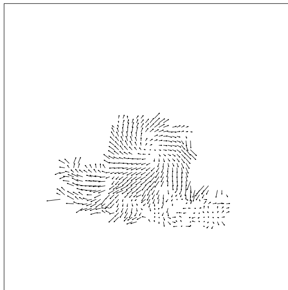
Fig.4 Optical flow using the algorithm of this work for translation and rotation synthetic image sequence.
