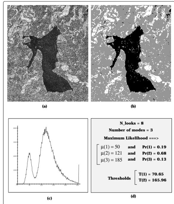
Figure 8: (a) Original RADARSAT SAR image (532x600), (b) Segmented image, (c) Histogram of filtered image and (d) Estimated parameters and thresholds.
